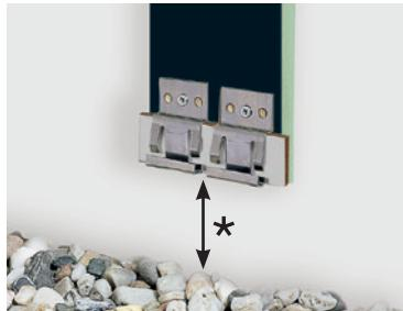
\*The wooden substructure distance to the water-bearing ground has to be 300 mm in minimum (if gravel-soil is given). In case of smooth grounds and strong weathering the splashing-water area increases up to 500 mm height.
